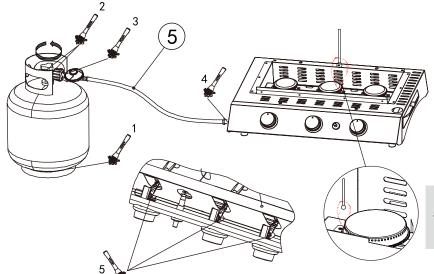
Consider to manually light the burner with a lit match as shown if failing to light with piezo ignition.
